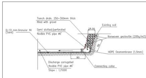
(b) Permanent drainage system detail
