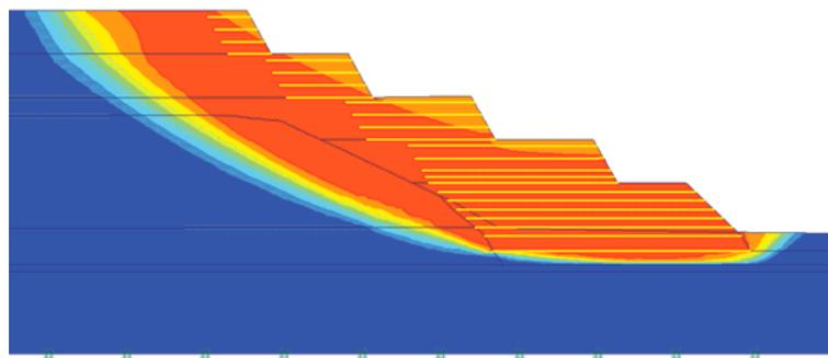
**Fig. 9:** RSS failure mechanism under seismic event (SF > 1.1)
