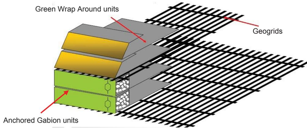
**Fig. 3:** Hybrid RSS structure components
