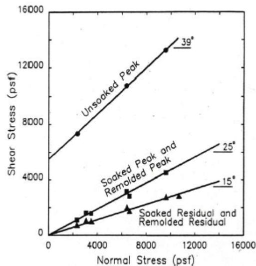
Fig. 2: Shear strength of soaked and unsoaked clay shale (Stark & Duncan, 1991)
