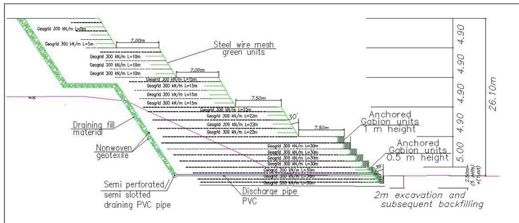
Fig. 6: Typical RSS section
