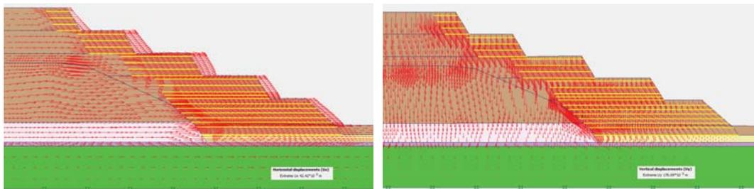
(a) Horizontal displacements after seismic event      (b) Vertical displacements after seismic event
