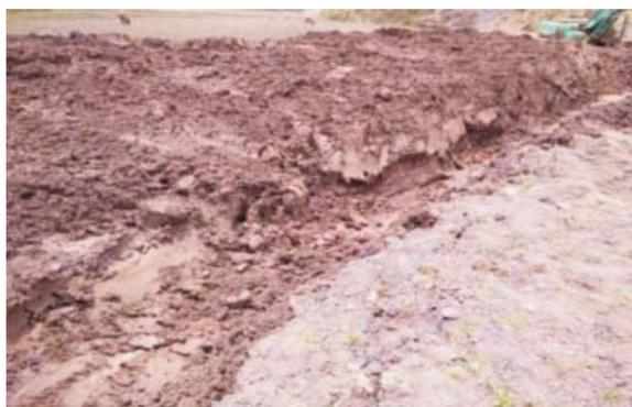
**Fig. 1:** Saturated clay shales
